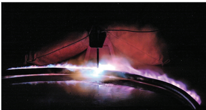
Dissipating Arcing Energy within Arc-Resistant Jacket
